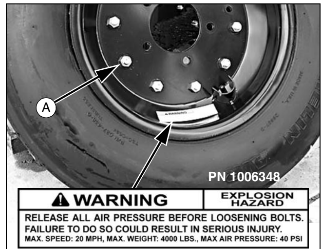
Figure 9. Split Rim Tire Servicing
